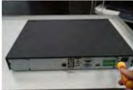
Figure 2-6 Removing the NVR Cover
