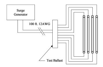
Fig. 1. Test circuit of electronic ballasts with no additional SPD protection applied.
